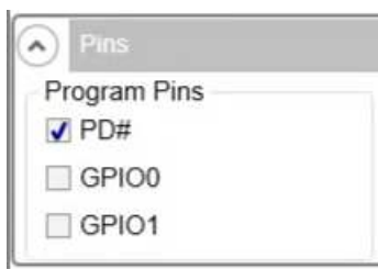
Figure 3-8. GPIO Pin Selection for SYSREF
