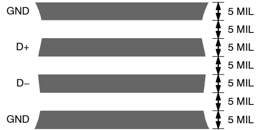
Figure 28. Arrangement of Signal Tracks
