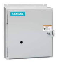
Non-reversing NEMA contactor, Size 2, Three phase full voltage, Contactor amp rating 45A, 3 wire (NO aux included), 208VAC 60Hz coil, Non-combination type, Enclosure NEMA type 12, Dust/drip proof for indoors, Extra-wide enclosure
