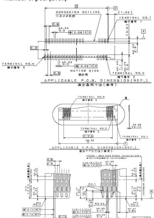
Note 2) To improve reliability of pitch direction positioning accuracy +0.05 -0.01 is recommended for dimension D.
