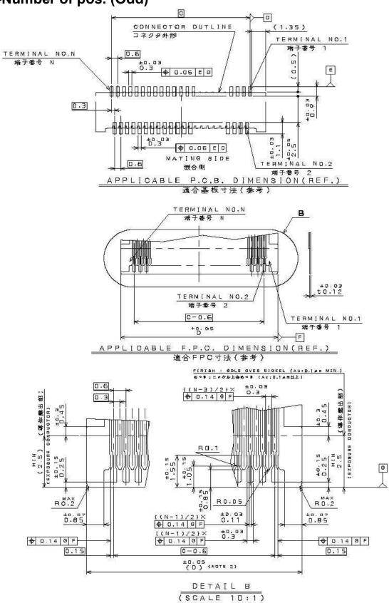
Note 2) To improve reliability of pitch direction positioning accuracy +0.05 -0.01 is recommended for dimension D.
