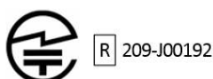
Figure 11.2. The Certification Mark to be Placed on the Outside Surface of the Host Equipment
