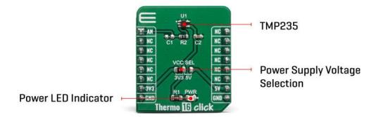
The TMP23X devices are a family of precision CMOS integrated-circuit linear analog temperature sensors with an output voltage proportional to temperature engineers can use in multiple analog temperature sensing applications. The TMP235 temperature sensor have an accuracy from 0°C to 70°C of  $\pm 1.25$ °C and provides a positive slope output of 10 mV/°C over the full -40°C to +150°C temperature range.
