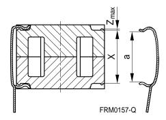
$F_{min}$ : Extension of clamp from a to  $a_2 = X_{min}$  $F_{max}$ : Extension of clamp from a to  $a_1 = X_{max}$
