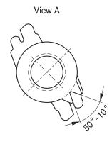
Hole arrangement View in mounting direction
