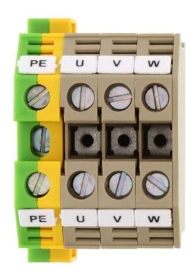
Four-wire motor-connection block, Screw connection, Mounting type:Mounting rail TS 35/7.5 and TS 32, Rated cross-section: 10 mm², Colour: Multi-coloured
