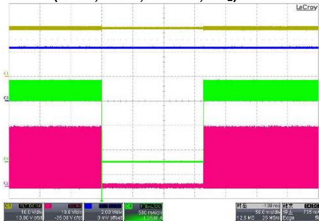
LED open protection(Vin=20V, 3LEDs) (Y-Vin, R-SW, B-VSET, G-I L )
