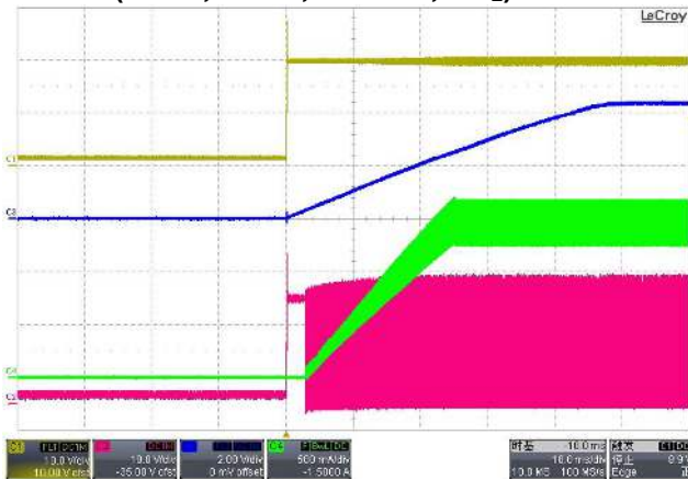
Soft Start waveform (Vin=20V, 3LEDs, C4=10nF) (Y-Vin, R-SW, B-VSET, G-I L )
