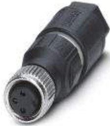
Sensor/actuator connector, female connector, straight, 3-pos., M8, QUICKON-ONE, metal knurl, maximum cable diameter of 5.0 mm
