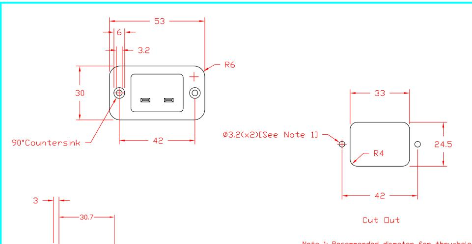
Note 1: Recommended diameter for thru-hole (screw/nut combination) hardware mounting method. Other methods will require holes with different dimensions and parameters.
