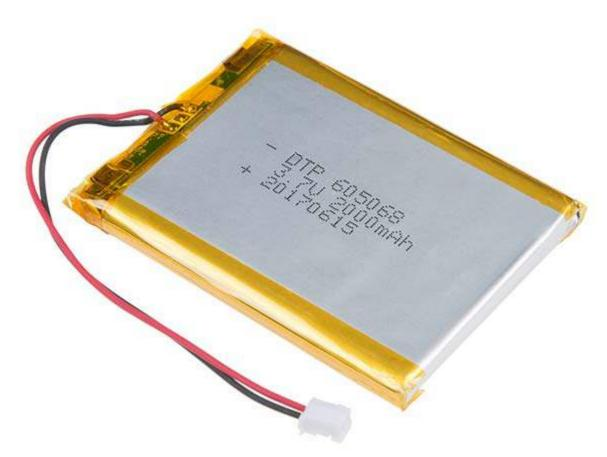
**Description:** These are very slim, extremely light weight batteries based on Lithium Ion chemistry. Each cell outputs a nominal 3.7V at 2000mAh! Comes terminated with a standard 2-pin JST-PH connector - 2mm spacing between pins. These batteries require special charging. Do not attempt to charge these with anything but a specialized Lithium Polymer charger.
