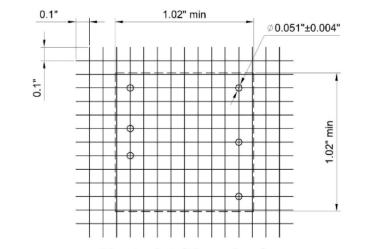
Unit: inch PIN tolerance:  $\pm 0.004$  Tolerance: X.XX  $\pm 0.02$  X.XXX  $\pm 0.01$
