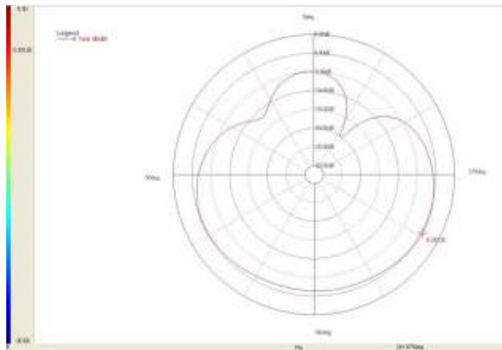
2D Radiation Pattern X-Y Plane 2450MHz
