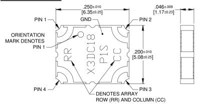
Dimensions are in Inches [Millimeters] X3DC18P1S Mechanical Outline
