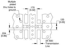
Dimensions are in Inches [Millimeters] X3DC18P1S Mounting Footprint
