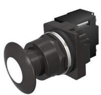
30mm BlackMax, Epoxy Coated Corrosion Resistant Complete Metal Unit Illuminated Push-Pull Operator Full Voltage, 6V AC/DC Incandescent Lamp Mushroom Head Cap Small 1 3/4" (44.5 mm) Metal, Black with White Lens 3 Position Momentary UL Listed, CSA Certified NEMA 1,3,3R,4,4X,12,13 & Automotive Standards
