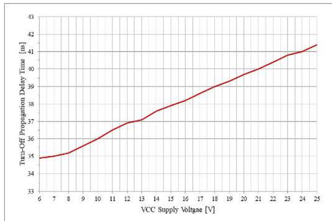
Figure 47. Turn-off Propagation Delay vs. V_{CC} Supply Voltage
