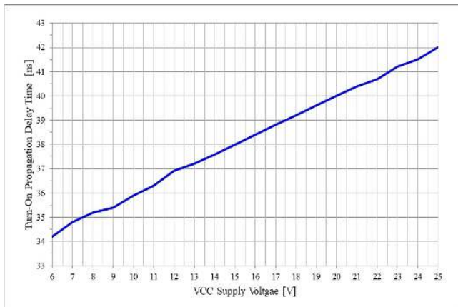
Figure 46. Turn-on Propagation Delay vs. V_{CC} Supply Voltage
