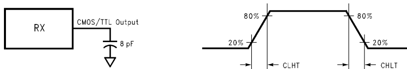
Figure 7. LVC MOS/LVTTL Output Load and Transition Times
