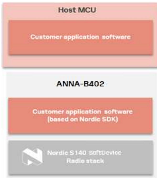
Figure 2: ANNA-B402 software structure and available software options
