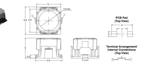
Note: Unless otherwise specified, a tolerance of  $\pm 0.4$  mm applies to all dimensions. No terminal numbers are indicated on the Switches.
