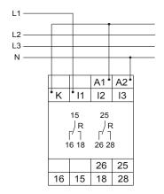
Measuring range 10A, supply voltage 230V AC
