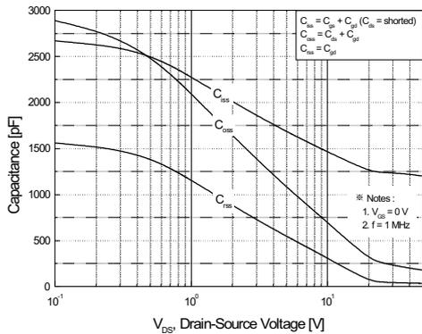
Figure 5. Capacitance Characteristics
