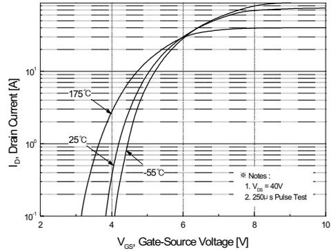
Figure 2. Transfer Characteristics
