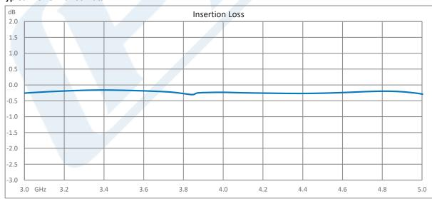
Click the following link (or enter part number in "SEARCH" on website) to obtain additional part information including price, inventory and certifications: Circulator with 18 dB Isolation from 3 GHz to 5 GHz, 10 Watts and SMA Female PE83CR1033
