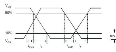
Switching Time Waveforms
