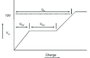
Basic Gate Charge Waveform
