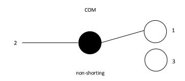
Type of Schematic: SPDT
