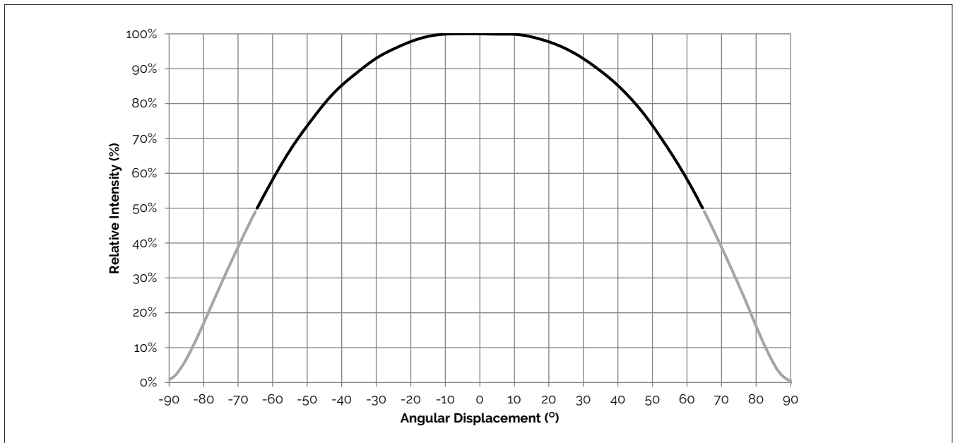
Figure 20: Typical Spatial Radiation Pattern
