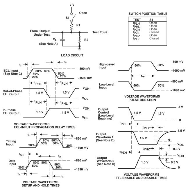
NOTES: A.C. includes probe and jig capacitance.
