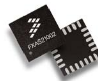
24 QFN 4 mm x 4 mm x 1 mm Case 2209-01
