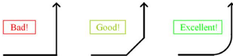
Figure 5-13: Examples of Turns in Trace Routing
