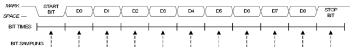
Figure 26.4. 9-Bit UART Timing Diagram
