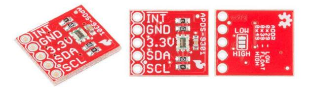
The APDS-9301 Ambient Light Sensor Breakout is an I<sup>2</sup>C-compatible luminosity sensor board that converts light intensity to a digital output signal. This breakout is fairly simple and has been specifically designed with only a few ancillary passive components in addition to the ADPS-9301 IC itself. All readings are returned to your chosen microprocessor in lux, providing precise Illuminance measurement under diverse lighting conditions.
