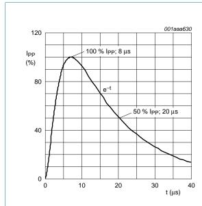
Fig 1. 8/20  $\mu s$  pulse waveform according to IEC 61000-4-5
