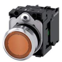
Illuminated pushbutton, 22 mm, round, metal, shiny, amber, pushbutton, flat, momentary contact type, with holder, 1 NO, LED module with integrated LED 230 V AC, screw terminal
