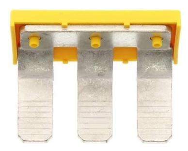
External insulated cross-connector, No. of poles: 3, Mounting type: Plug in, Width: 57.04 mm, Rated current: 150 A; Colour: Yellow
