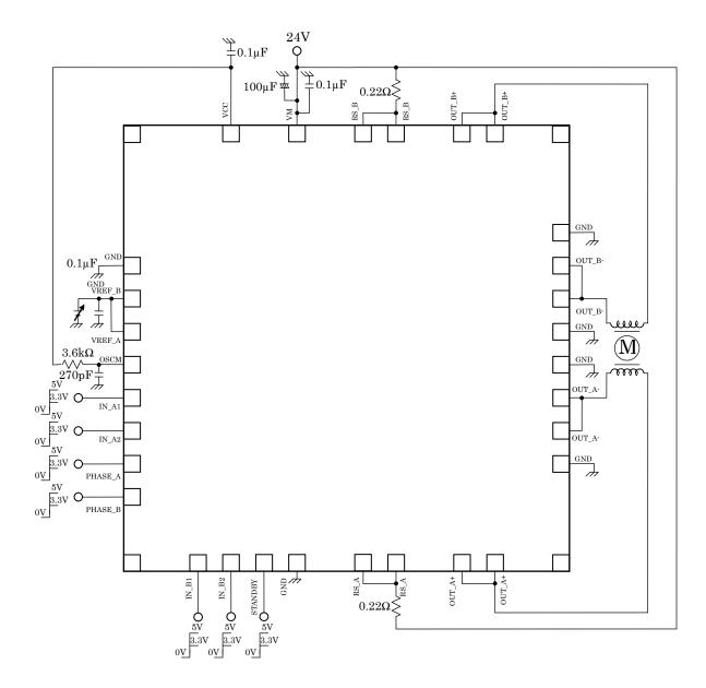
Note: Bypass capacitors should be added as necessary. It is recommended to use a single ground plane for the entire board whenever possible.
