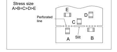
to varistor placement, consider the board breaking method as well.
