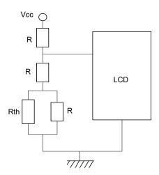
Temperature compensation (RF circuit)
