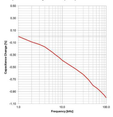
Test Equipment: E4991A or equivalent
