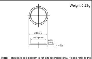
Note: This bare cell diagram is for size reference only. Please refer to the tab configurations at the end of this section for available tabs.
