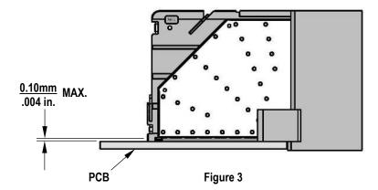
There should be no broken stand-offs along the perimeter of the part (an indication of over-pressing).
