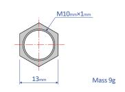
Note: When attaching, make sure that the side without a bearing chamfer is the impact surface.
