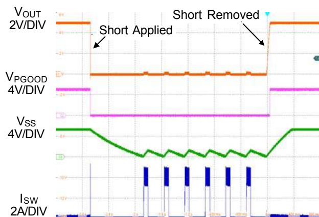
Figure 3. Short-Circuit Protection and Recovery
