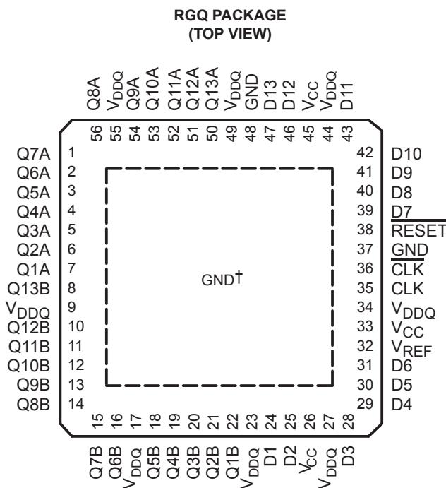
† The center die pad must be connected to GND.
