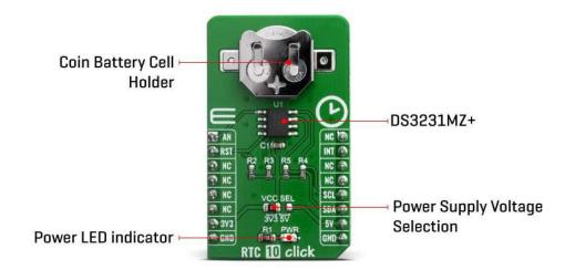
In addition to the DS3231M, RTC 10 click is equipped with the button cell battery holder compatible with the 3000TR batteryholder, suitable for 12mm Coin Cell batteries. By utilizing an automatic backup switch, the IC is able to use an external battery power source when there is no power supply on its main power terminals, thus allowing for uninterrupted operation.
