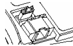
Figure 7: Slave Setting for Vertical iDiskOnChip 40-Pin Connector
