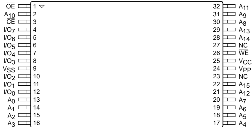
TSOP Package (Reverse Pinout) (TR, HR)
