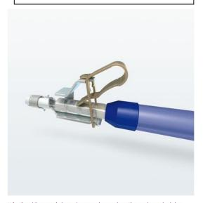
Whether it's a push-in spring or a leg spring, the spring principle makes for quick, tool-free conductor connection. Simply insert the solid conductors and conductors with ferrules into the push-in terminal point and release using a screwdriver. When connecting and releasing finely stranded conductors without ferrules, the terminal point can also be opened using a screwdriver. AC wire connection instruction
