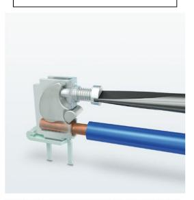
Cable routing and actuation of the terminal block screw on one level – front screw connection for narrow device fronts and PCB racks. The conductor is reliably clamped by the force-increasing swiveling movement of the angled pressure plate.
