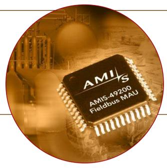
In most applications, the AMIS-49200 can be used as a replacement for the  $\mu$ SAA22Q. Some external component values may have to be changed but, in most cases, the layout of the circuit board will not have to change.
