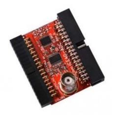
This is an extension module for iCE40HX1K-EVB. It is meant to add fast Analog-Digital-Converter (ADC) functionality to the main board. You can use up to 4 x iCE40-ADC with the same iCE40HX1K-EVB (up to 2 x iCE40-ADC when you have iCE40-IO connected to the same bus).
