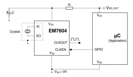
The RC filter is composed of a capacitor (C) and resistor (R) implemented per example by a  $1k\Omega$  resistor and a  $10\mu F$  capacitor. The resistor and the capacitor can be adapted if needed.
