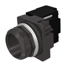
30mm BlackMax, Epoxy Coated Corrosion Resistant Complete Metal Unit Illuminated Indicator Light Transformer type, 240V AC Incandescent Lamp, BA9s Less Lens UL Listed, CSA Certified NEMA 1,3,3R,4,4X,12,13 & Automotive Standards
